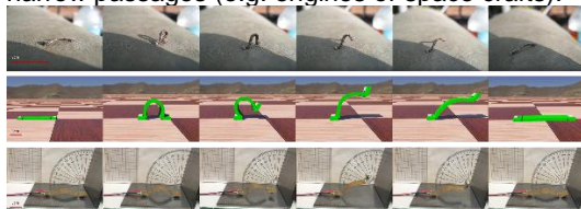
[top] Real Inchworm walking, [middle] Inchworming robot implemented in simulation (Webots), [bottom] Real inchworm robot prototype
