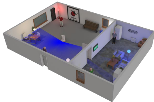
Fig.1 : The pilot use case in Webots simulator. A TIAGo Iron robot moves in an apartment while avoiding obstacle using its lidar sensor.
