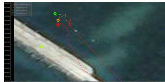
Field test; green: boat sender; orange: GPS position; red: estimated position
