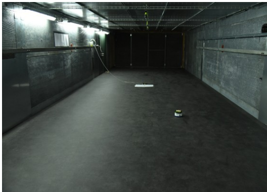
Illustration: A KheperaIV running an algorithm in the wind tunnel. The source is located above the white sheet of paper in the back, 10 cm above the ground. The wind comes from the background wall.
