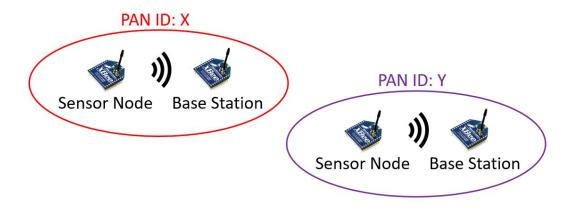
In the Part 3 folder, open the file receiver.ino. Take a look at the code and notice that another serial line is initialized in the setup (Serial3). This serial line is connected to the Xbee and is used to transmit and receive data through wireless communication. At line 33 **change the PAN ID by substituting the number 2019 with the number of your computer** in the computer room (eg., Serial3.print("ATID 3\r"); ). Upload the code to the board that you are going to use as base station.
