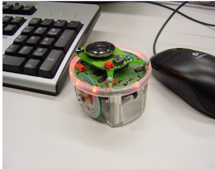
Figure 1: Close-up of an e-puck robot.
